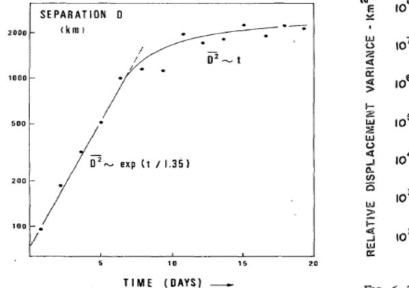
FIG. 8. Root mean square separation of the original pairs of balloons released during the EOLE experiment, as a function of time after launch.
