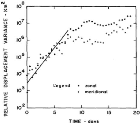
FIG. 6. The mean-square relative displacement components for midlatitudes releases on a log-linear scale. The straight line indicates an exponential region.
