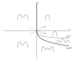
Tricritical point corresponding to the normal form  $s(m) = -m^6 - \frac{3b}{2}m^4 - 3am^2$ .
