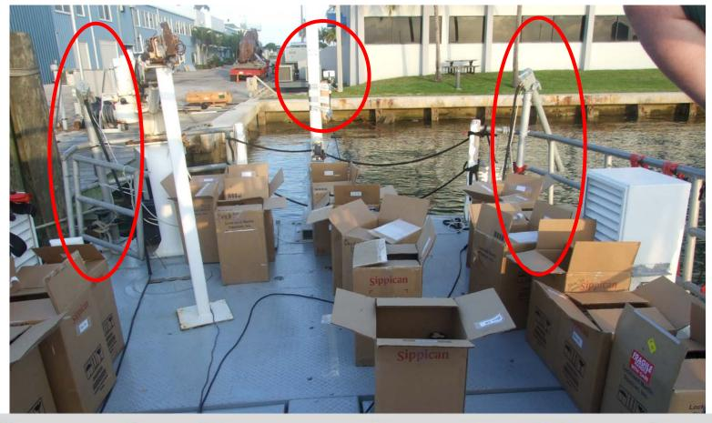
Allows simultaneous launch of 3 probes
