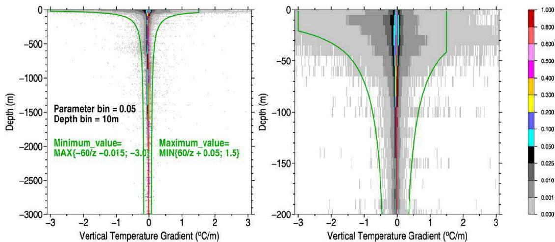
Fig. 4.18: Normalized temperature vertical gradient histogram. For each level the number of the data in each bin is divided by the number of data for the most populated bin. The min-max vertical gradient limits shown in green are subjectively approximated by the reciprocal function of depth
