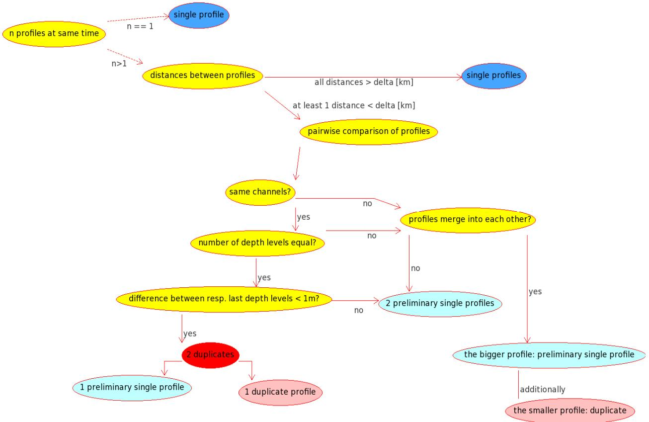
*Fig. 4.8: Schematic diagram to explain the elimination of duplicate observational data. A profile classified as “preliminary single profile” in one pairwise comparison may be identified as a duplicate profile in a later pairwise comparison.*
