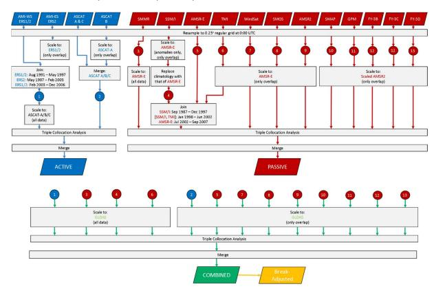
Figure 13: Overview of the processing steps in the ESA CCI SM product generation (v07.1): The merging of two or more data sets is done by weighted averaging and involves overlapping time periods, whereas the process of joining data sets only concatenates two or more data sets between the predefined time periods. The join process is performed on datasets of each lines and on datasets separated by comma
