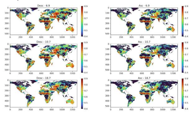
Figure 6: Visualized correlation of nighttime (descending) and daytime (ascending) observations against SMAP Level 4 SM, for C- (6.9 GHz), X- (10.7 GHz), and Ku-band (18.7 GHz) from AMSR2, using LPRMv7.0.
