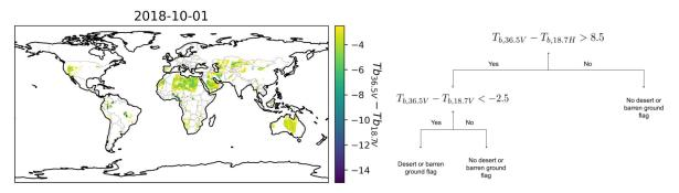
Figure 9: (left) Barren ground and related desert regions are clearly visible when using the first step of the snow/frozen flag without the correction for low physical temperatures. (right) Final decision tree for the barren soil flagging.
