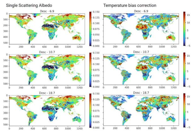
Figure 4:  $\omega$ , the single scattering albedo, and dT, local bias correction of the land surface temperature, results from the optimization for C-, X- and Ku-band.
