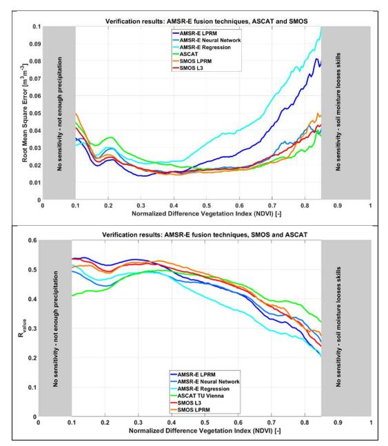
Figure 8: Triple collocation analysis (TCA: top) and  $R_{value}$  results (bottom) for several soil moisture datasets, including SMOS LPRM and AMSR-E LPRM, for changing vegetation density (NDVI). Based on (van der Schalie et al., 2018).
