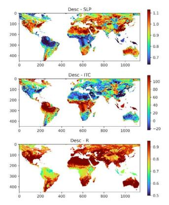
Figure 3: Slope, Intercept and Correlation of Ka-band against ERA5-Land temperature. Note that the interpolation over the tropical region in Africa has since been improved.
