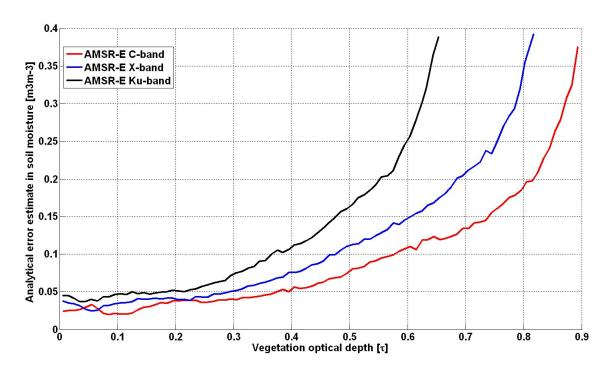
Figure 7: Error of soil moisture as related to the vegetation optical depth for 3 different frequency bands (from Parinussa et al., 2011).
