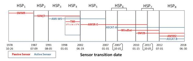
Figure 17: Potential break times in the ESA CCI SM v04.4 (COMBINED) product- corresponding to changeovers in the blended sensors, building the homogeneous (sensor) sub-periods (HSP).
