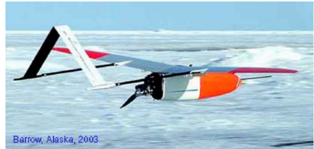
Fig. 4. An Aerosonde UAV in a landing approach during one of the Barrow, Alaska-based missions.
