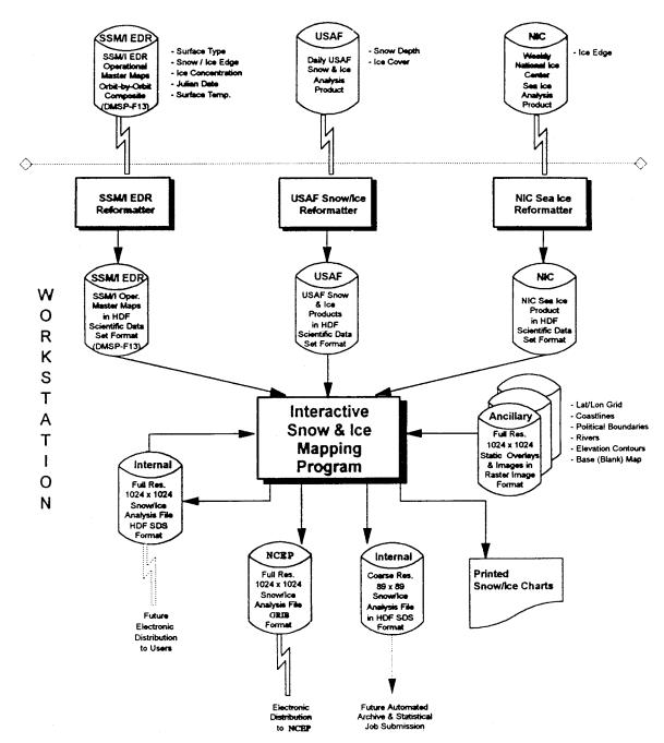
Figure 4. Flow chart showing data processing of IMS
