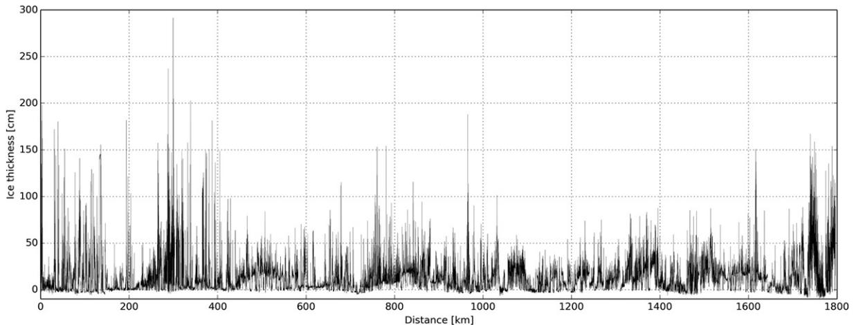
**Fig. 5.** Sea ice thickness profile measured with the SEM at the bow of RV Lance from March 18 to 27, 2014. The location of the 1800 km long track is shown in Fig. 7. The thickness measurements were spatially averaged over 25 m distances according to the GPS position of RV Lance.
