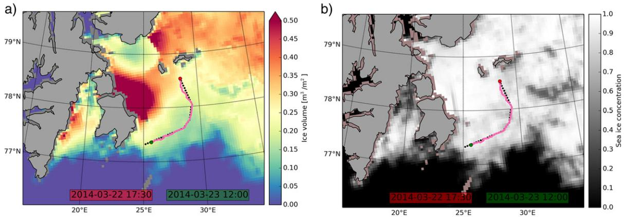
**Fig. 9.** Example of optimized route suggestion from the forecast system (black dotted line) and actual track of RV Lance (magenta line) overlaid on sea ice thickness (left) and concentration (right) from the forecast model. The mean sea ice thickness per grid cell is the product from the model effective sea ice thickness  $h_i$  and concentration  $C$  which equals the sea ice volume per unit area.
