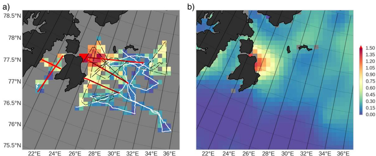
**Fig. 7.** Ground (left) and SMOS sea ice thickness (right) color-coded in meter. The ground data consists of SEM (white) and HEM (black) and ALS (red) measurements block averaged with 12.5 km grid resolution. The SMOS map represents a temporal average over the period March 19 to 26.
