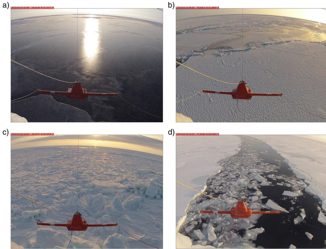
**Fig. 4.** Example ice conditions and EM thicknesses measured at the bow of RV Lance: a) Dark nilas of 2–4 cm thickness, b) grey white level ice of 17 cm thickness, c) pressure/rubble ice field of 3.4 m thickness, d) navigating through a lead with a mean thickness of 17 cm.
