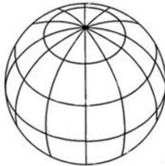
Figure 5. Convergence of longitude lines produces shrinking of 1^\circ \times 1^\circ grid cells toward the poles.
